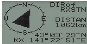
Compass display shows the direction to the received station
